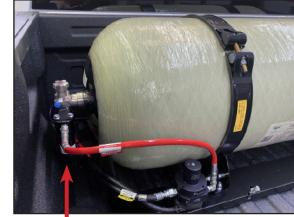
Bleeder Valve Plug on Trucks. In bed of truck under cylinder cover.
