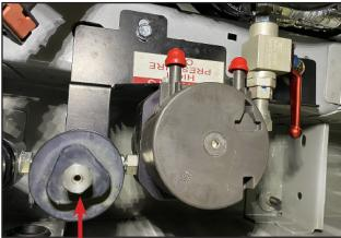
Bleeder Valve Plug on Transit. Under the vehicle and driver door.
